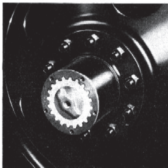
Fig 46—Shaft to Hub Adjustment
