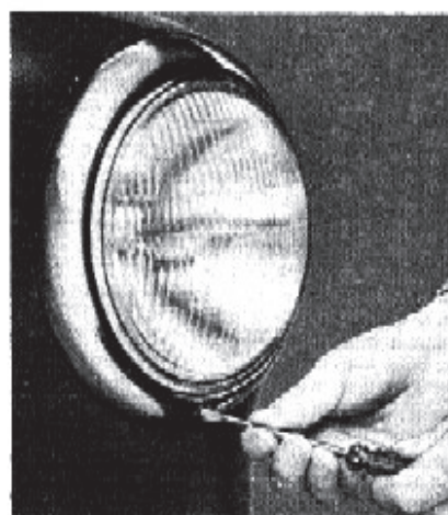
Fig. 58—Removing Headlamp Rim
