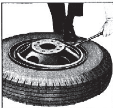
Fig. 70—Installing Clamp Ring
